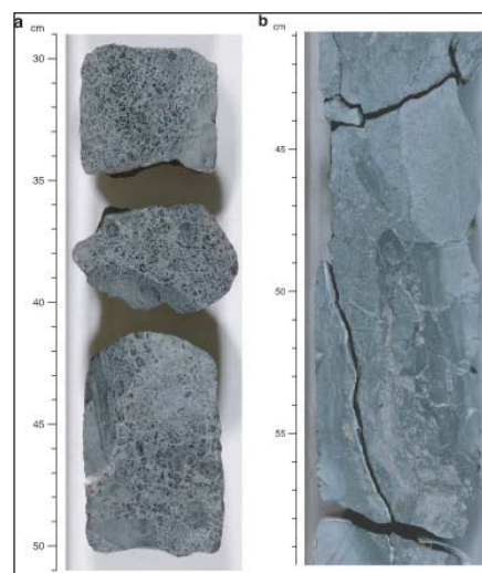
Figure 3 (a) Example of the mineralized volcanic breccia characterized by variably altered clasts of hyaloclastite in a sulfide matrix (interval 309-1256D, 122R-1, 29–51 cm). (b) Sulfide impregnated dike margin breccia (interval 309-1256D-140R-1, 42–58 cm).
