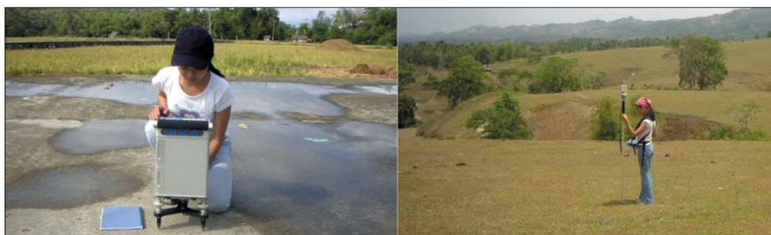
Figure 1 Ground gravity (left) and magnetic surveys (right) were conducted on the islands of Tablas, Romblon and Sibuyan.
