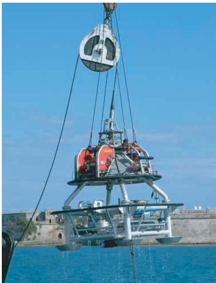
Figure 1. Photo of the observatory off board of the moto-pontoon "Mazzarò" during final trials before deployment of offshore Eastern Sicily.
