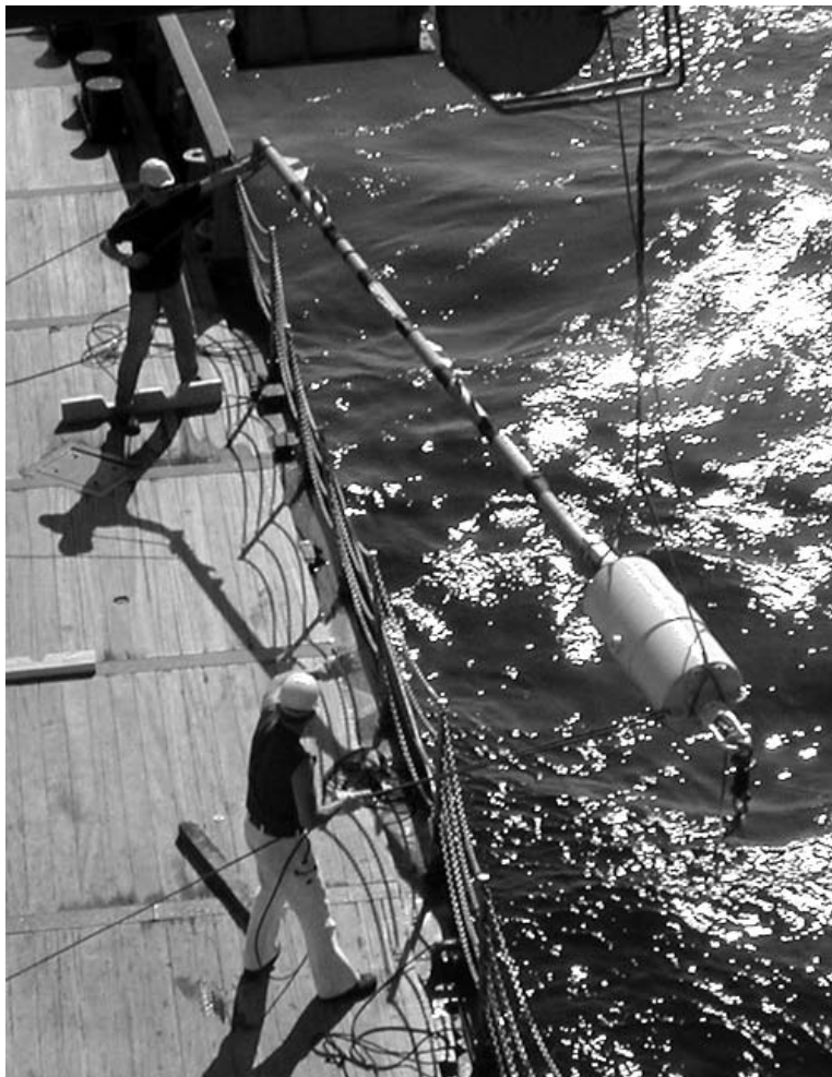
Figure 2. Deployment of the heatflow probe during the LuckyFlux cruise. The 1-Ton weight holds the acquisition and power supply system. The thermistors protruding from the 7-m long probe are also visible.
