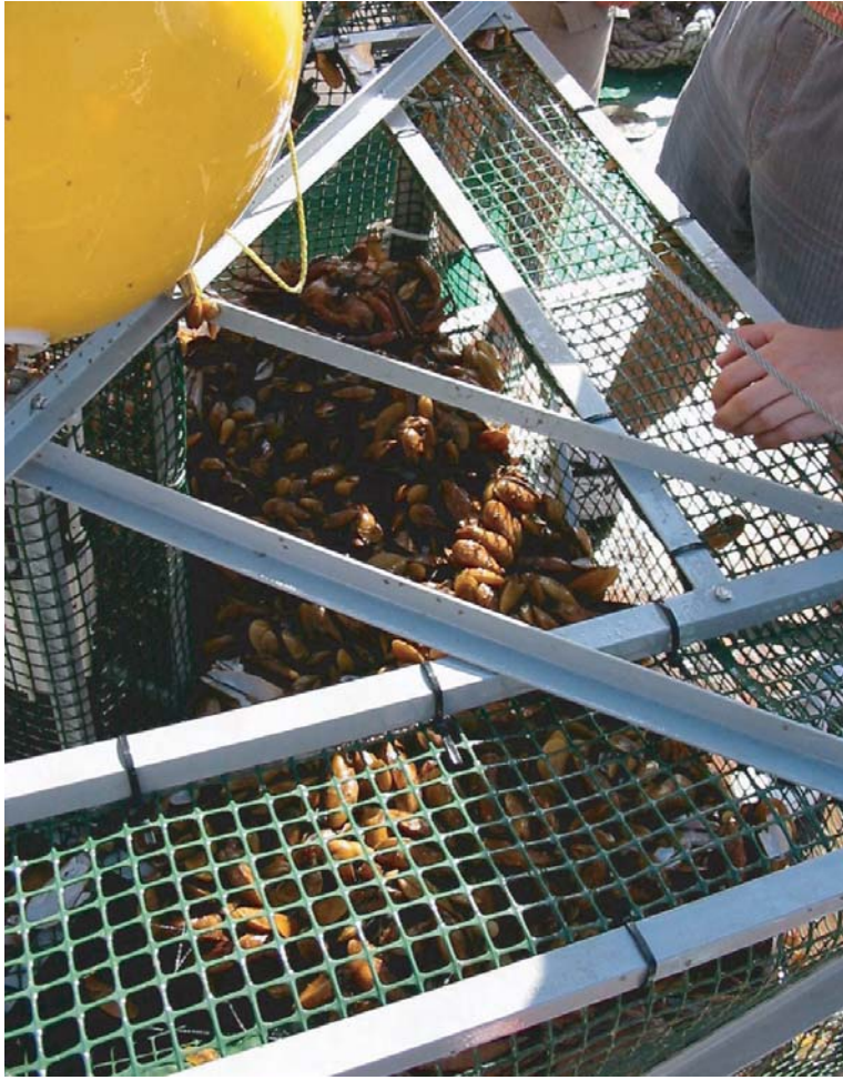
Figure 2. Cage at the time of recovery on board the R/V Arquipélago. The broken shells date back to when the cage was loaded using the ROV.
