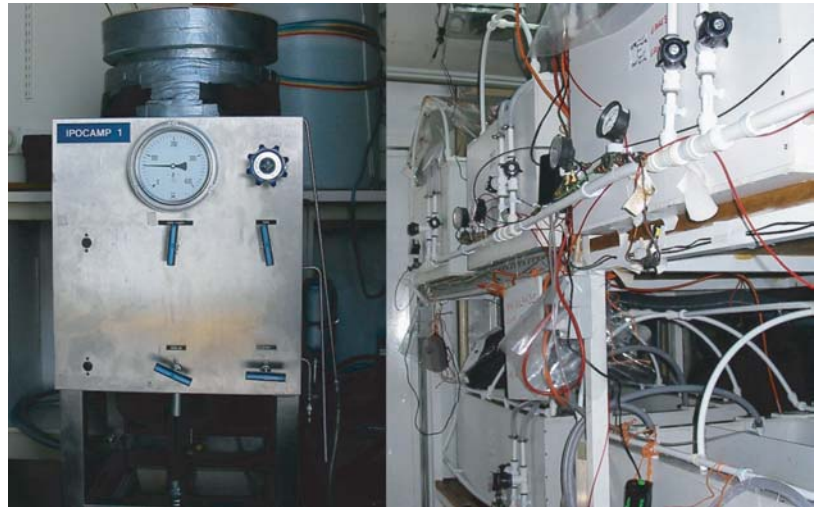
Figure 4. Interior view of LabHorta laboratory complex showing high pressure chamber (IPOCAMP 1 - Université Pierre et Marie Curie, Paris) and stock and experimental aquaria.
