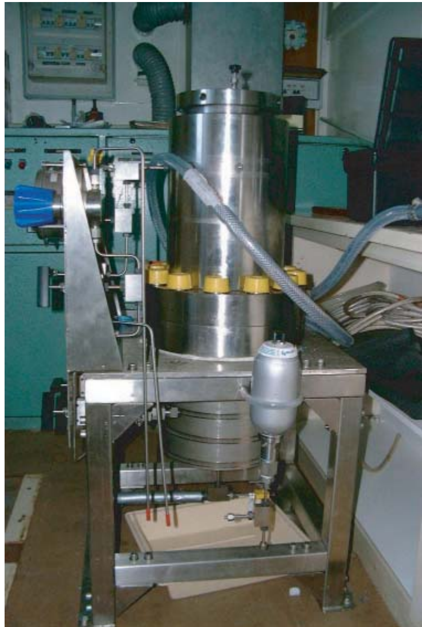
Figure 3. The IPOCAM P flow through pressure chamber.
