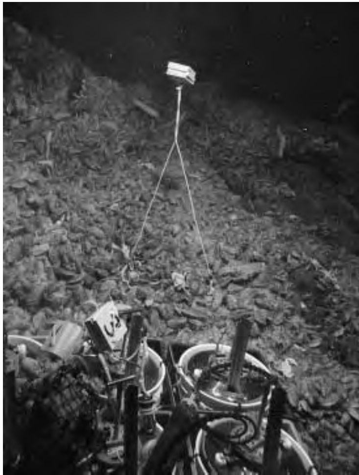
Figure 2. Temperature probe deployment configuration, Train Station 1999.
